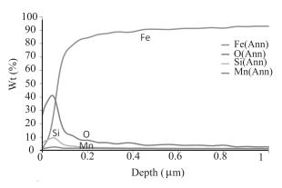
**Fig.5.** GDOES depth profiles of the annealed sheet containing rolled-in scale.
