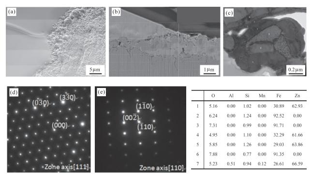
Fig.8. Cross sectional analysis of galvanized sample by TEM/EDS and SAED.
