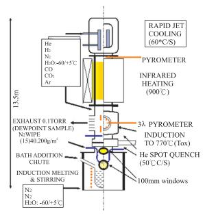
Fig.1. Schematic diagram of the galvanizing simulator.
