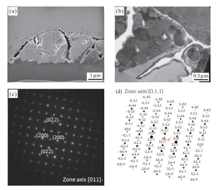
Fig.7. The microstructure analyses of TEM/SAED of the annealed rolled-in scale area.
